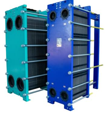
Gasket plate heat exchanger's temperature bearing range is between -40-180°C, which is depending on gasket material. It's qualified of the process of heat exchanging and waste heat recovery in district heating system. Its volume capability is variable by simple increase or decrease the number of the plates.
