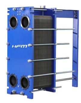
Gasket plate heat exchanger's temperature bearing range is between -40-180°C, which is depending on gasket material. It's qualified of the process of heat exchanging and waste heat recovery in data center. Its volume capability is variable by simple increase or decrease the number of the plates.
