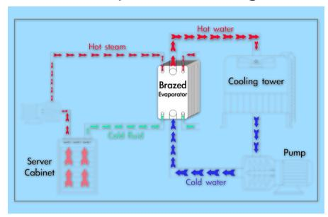
In the first graphic, the hot air within the cabinet is delivered to the radiator, thermal energy is transmitted to the water, in this circle, the brazed heat exchanger keeps chilling hot water. On the other side, thermal energy passes through plates to the water of the other circle. There is few state transform of the fluid due to its high boiling point under proper design, which is called "Single-phase cooling".
