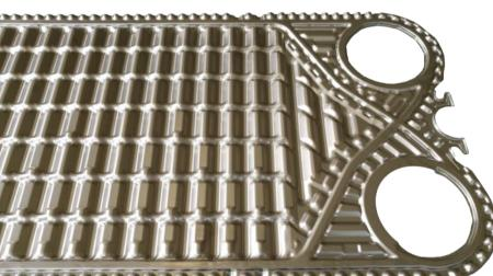
Given the viscosity of sugar is relatively high and the temperature is not too high, SS 316 is a good choice, EPDM is used for the rubber pad. The flow velocity of the low-pressure steam interface should be less than 50m/s. The logarithmic average is 42.5°C, which is greater than 10, the 8mm deep wide gap plates allow high velocity flow (up to 5mm diameter particles) going through without retention.
