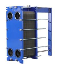
The Gasket plate heat exchanger is expandable and easy servicing. However, in terms of high concentrated sulphuric acid, gasket we only recommend Viton-G, and as show on the left, the sulphuric acid has to below 100 degrees celsius.
