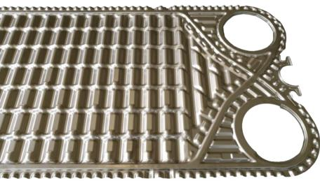
Plates with deeper corrugation means large diameter particles or high viscosity fluid could easily pass through. The 8mm deep wide gap plates allow pulp (up to 5mm diameter particles) going through without retention.
