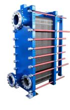
The Semi-Welded Plate Heat Exchanger, one side is sealed by laser welding, and the other side is sealed by gaskets. This increases maintainability, but allows the use of aggressive medium and higher pressure than the completely inflated model. This means that the heat exchanger can be used in the application of refrigerants
