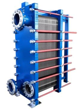
The Semi-Welded Plate Heat Exchanger, one side is sealed by laser welding, and the other side is sealed by gaskets. This increases maintainability, but allows the use of aggressive medium and higher pressure than the completely inflated model. This means that the heat exchanger can be used for evaporating ammonia.
