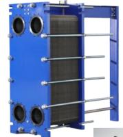
The Gasket plate heat exchanger is expandable and easy servicing. It is used in lowtemperature and lowpressure conditions, such as closed cooling water circuits.
