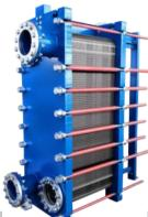
The Semi-Welded Plate Heat Exchanger, one side is sealed by laser welding, and the other side is sealed by gaskets. This increases maintainability, but allows the use of aggressive medium and higher pressure than the completely inflated model.
