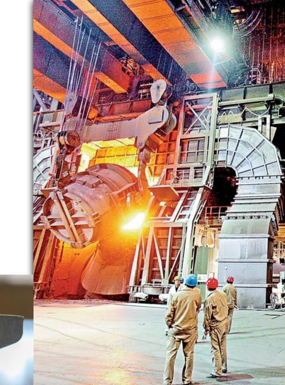
Steel is refined by melting iron ore. The production is roughly divided into sintering process, DRI (Direct Reduced Iron), steelmaking and continuous casting process of producing billets, and rolling process of making various steel materials. In addition, there are coking, oxygen production, hydropower, etc.
