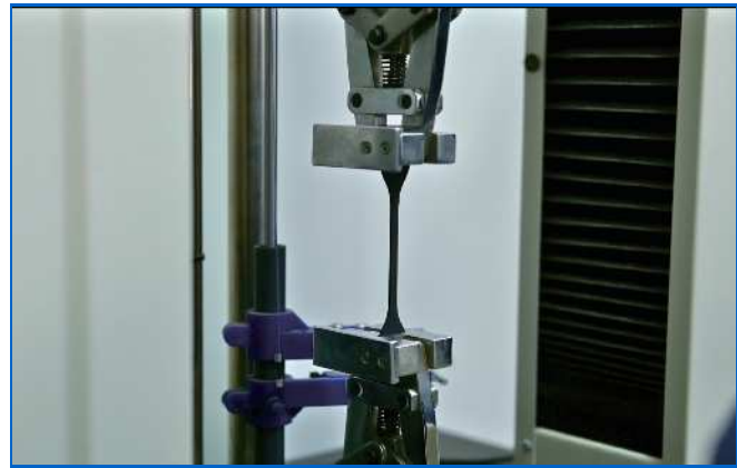
Tensile Testing of Gasket Material
