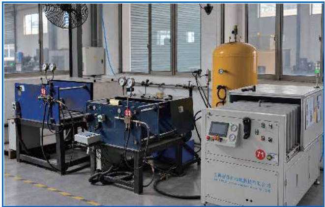
Pneumatic Pressure Testing of Brazed Plate Heat Exchangers
