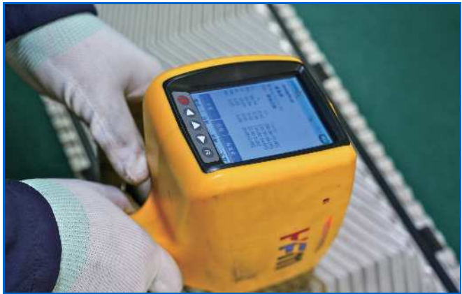
Positive Material Identification (PMI) on plate
