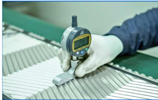
Plate Corrugation Depth Measurement
