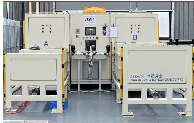
Vacuum Helium Leak Testing
