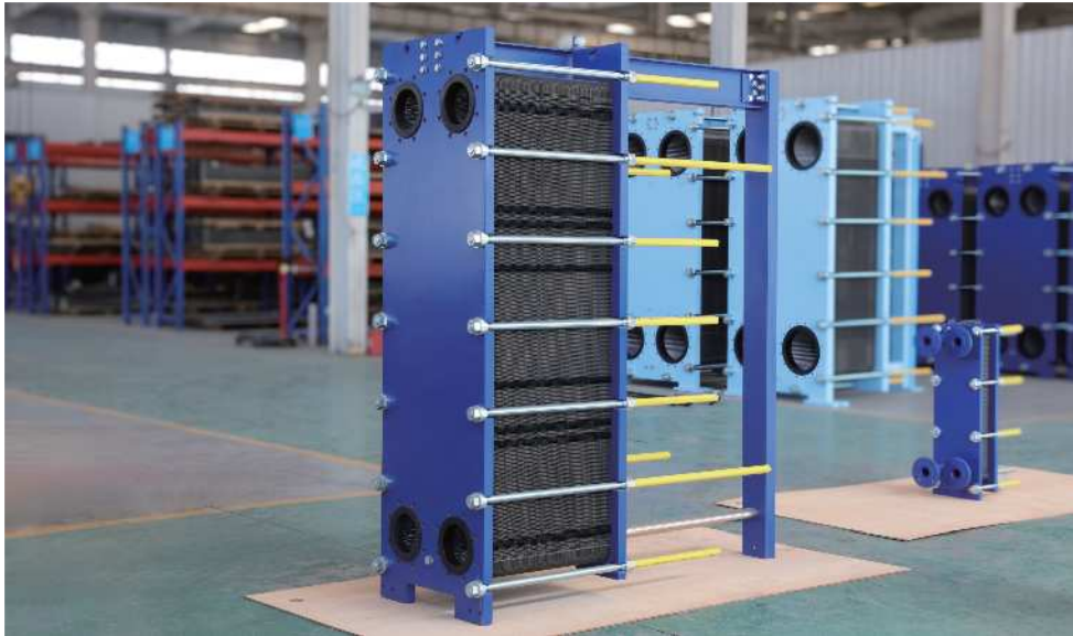
Inspecting and adjusting the tightening dimensions of a Plate Heat Exchanger
